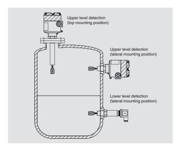
The vibrating level switch is usually installed on the side of the tank to detect the upper and lower liquid levels. If the vessel has no side openings, the limit level switch can also be mounted on the tank from above. A pipe extension is then often used to achieve the desired switch point. Installation on the underside of the tank is also possible.
