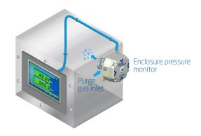
**Pressurization:** After purge is complete, the automatic leakage compensation valve (ALCV) controls the air supply to maintain a constant pressure inside the enclosure and compensate for any small leaks, thus preventing ingress of the outside atmosphere. The enclosure pressure is continuously monitored. The electrical equipment inside the enclosure can now be energised.
