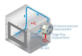
**Purge:** The SmartPurge Z supplies clean, dry instrument air to the enclosure at a high flow rate for a pre-set time, expelling any potentially flammable atmosphere remaining inside through the system relief valve. Enclosure pressure and purge flow are both monitored during this phase, and the electrical equipment inside the enclosure must not be energised.
