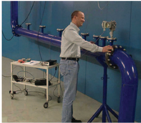
The systec testing facility determines the effect shortened inlet paths have on the deltaflow.
